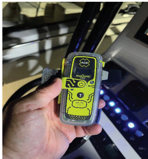
Figure 6: Photograph of the ACR ResQLink personal locator beacon found on the BIG STICK. Taken by U.S. Coast Guard Sector North Carolina Investigators on April 9, 2024.
