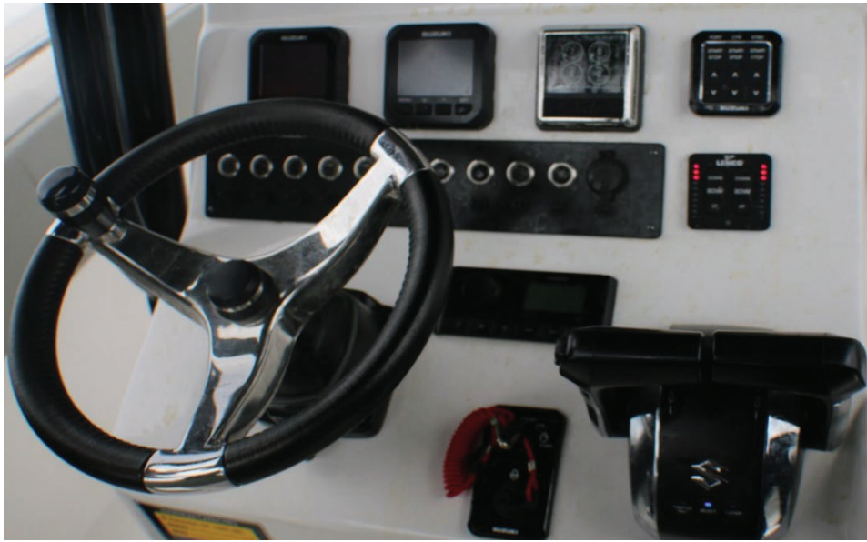
Figure 7: Photograph of the console of the BIG STICK, showing the lanyard-style engine kill switch to the right of the steering wheel. Captured by the USS SHERMAN boarding team on April 9, 2024.
